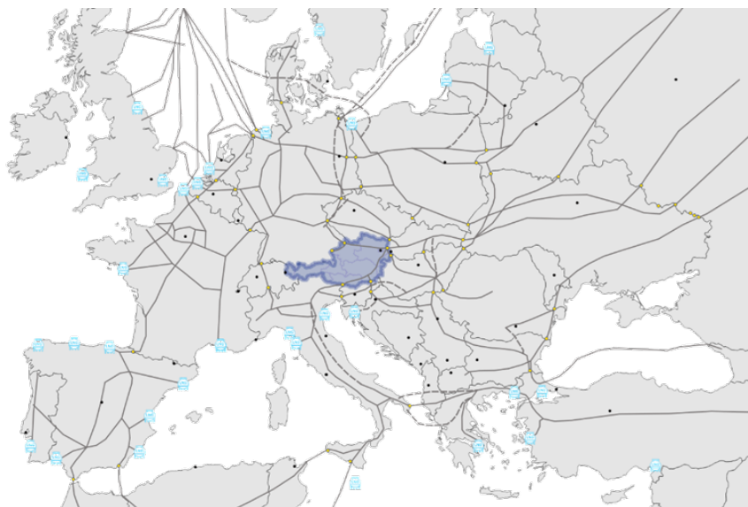
Figure 6: Pipeline network in Austrian surroundings
